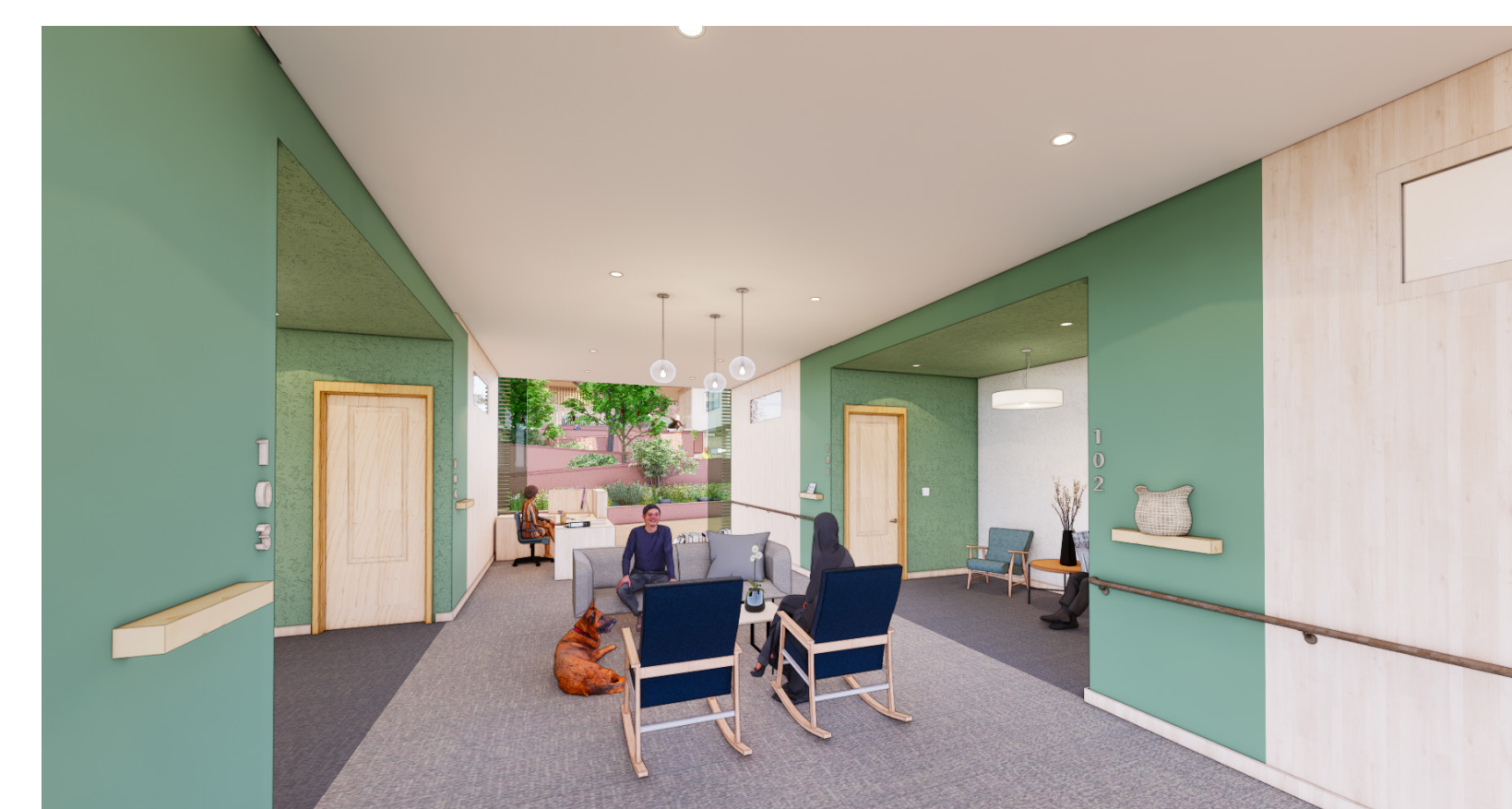
Color, texture, lighting, ceiling height and material change all help support non-verbal wayfinding and familiar objects initiate memory recall.
